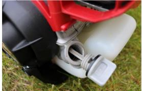
rather than filled at the same time as the fuel. The oil (just 100ml is needed) is directed to all components when the engine is at any angle — even upside down. Checking and changing oil (required every 50 hours) is also easy. The only additional maintenance which may require a workshop visit is checking the valve clearances on the engine. This is scheduled every 100 hours.
