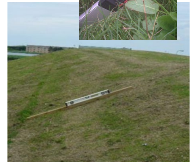
Consider using a straight edge in conjunction with slope measuring device when surveying longer spans
