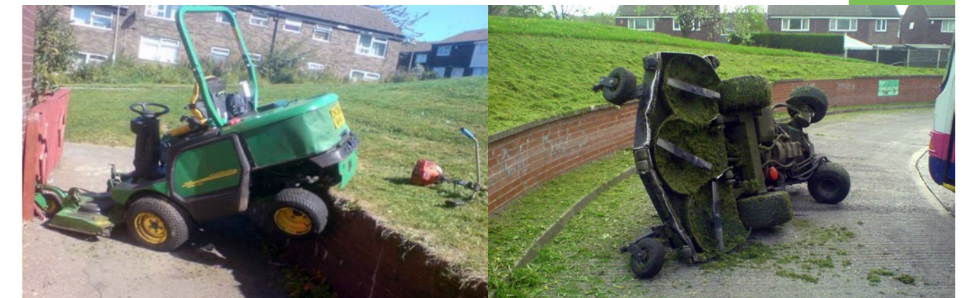
In the scenarios above, a pedestrian/walk-behind mower could have been used to maintain grass on the slope and avoid the need for a ride-on machine to be used adjacent to the retaining structure.
