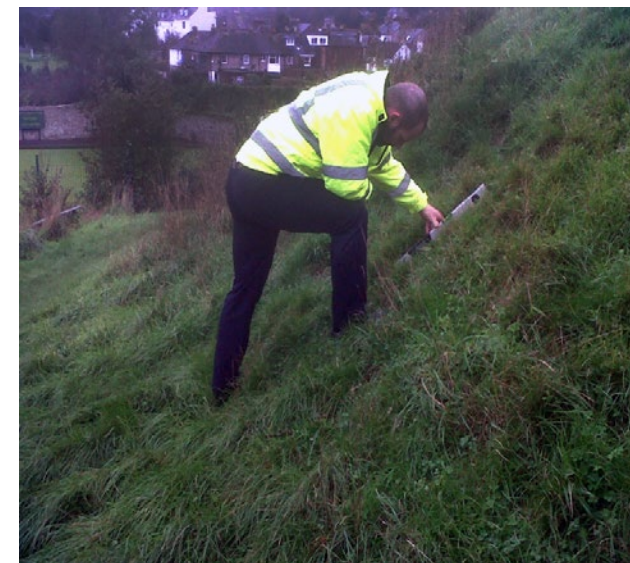
Person using angle measuring device on a slope
